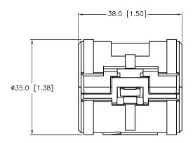
LOCKOUT DEVICE FITS A—SIZE (7/8") MINIFAST STRAIGHT TURCK FIELD WIREABLE CONNECTORS
