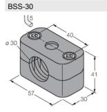
Mounting clamp for smooth and threaded barrel sensors; material:
