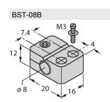
6947210 Mounting clamp for threaded barrel sensors, with dead-stop; material: PA6
