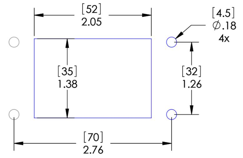
These devices shall be mounted on enclosures having adequate strength and thickness and with adequate spacing provided. Seal rating is based on mounting to a surface that is clean, flat and smooth.
