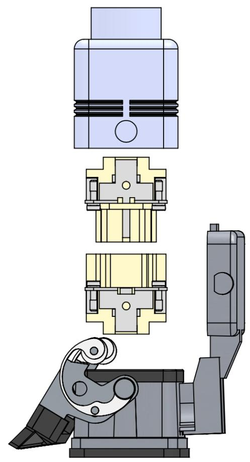
The Enclosures ensure IP66 protection (or IP65 for hinged cover versions) rating when mated and locked with the closing levers.
