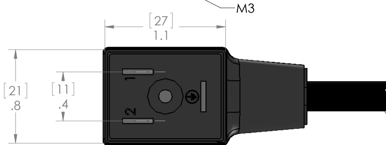
Gasket molded onto face of connector
