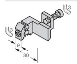
Mounting bracket for mounting magnetic field sensors on profile cylinders with external dovetail guide; cylinder diameter: 32...200 mm; material: Aluminum
