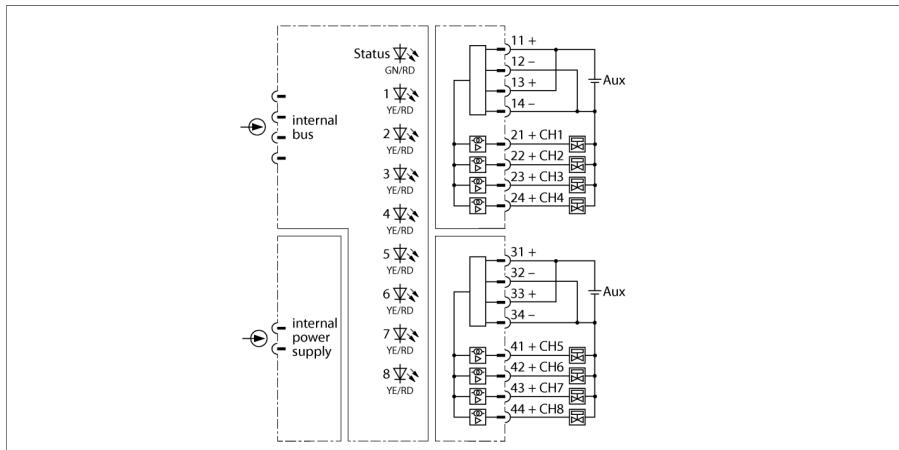
The output module DO80-N serves for connection of 24-VDC actuators. You can connect eight 24 VDC actuators such as valves or indicators with 0.5 A to it. The actuators are not powered via the module, but via a reverse-polarity protected auxiliary energy which is fed separately via the terminals to the channels 1 ... 4 (group 1) and 5 ... 8 (group 2). To increase the load, the outputs can be connected in parallel within a group. Both output circuits are galvanically isolated from each other.
