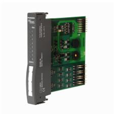
The digital input module DI80-N serves for connection of eight 3-wire PNP/NPN sensors (IEC 61131, Type 3). The sensors are not powered via the module, but via a reverse-polarity protected auxiliary energy which is fed separately via the terminals to the channels 1 ... 4 (group 1) and 5 ... 8 (group 2). The input groups are galvanically isolated from each other.
