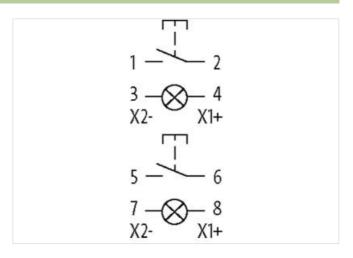
N/C1 Male PIN 1: N/C1 PIN 2: (X2/-)PIN 3: PIN 4: (X1/+) N/C 2 PIN 5: N/C 2 PIN 6: PIN 7: (X2/-)**PIN 8:** (X1/+)
