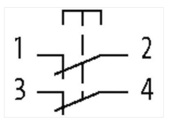
Male PIN 1: N/C1 PIN 2: N/C1 PIN 3: N/C 2 PIN 4: N/C 2
