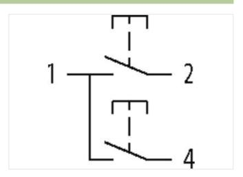
Male PIN 1: N/O 1/2 PIN 2: N/O 1 PIN 3: n.c. PIN 4: N/O 2
