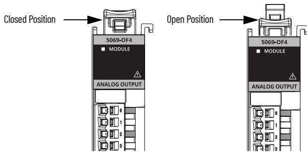
5. Align the interlocking pieces of the module with the device on the left. The top interlocking pieces engage first.
