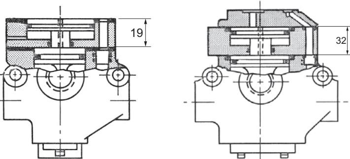
The adapter "PB" is used as an auxiliary piston to increase the actuation force.
