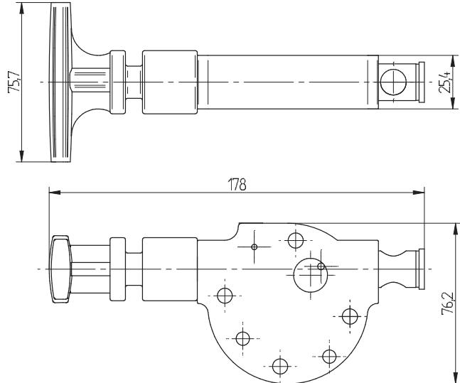
The adapter "LOX" ensures a pneumatic isolation of energy sources according to EN1037.
