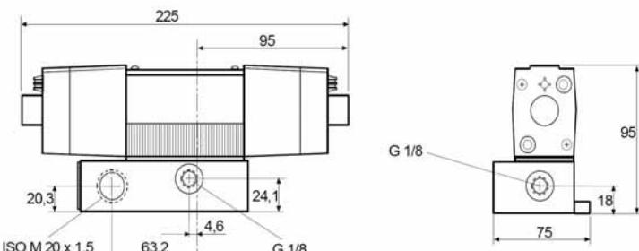
The double magnet solenoid pilot valve "CV1" allows for a controller via electrical impulses.
