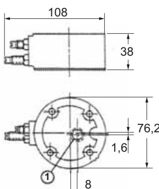
The switch-on / switch-off delay delays the "Switch-on time" (leaving the safe default position) of the ROSS poppet valves by means of mechanical flow restriction and differential pressure link. The adapter is an optional module between a ROSS poppet valve and an arbitrary controller.
