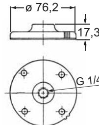
The pneumatic actuation comprises a cap attachment for the valve with an arbitrary connection thread for the control air connection.
