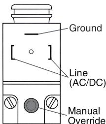
If power is supplied by a transformer it must be capable of handling the inrush current without significant voltage drop. See *Valve Specifications* on page 2 for information on inrush current.
