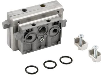
Different size ISO valves can be used in the same manifold installation by means of transition module. The inlet and exhaust ports of two different size manifold stations are connected by means of a transition module installed between the two stations.
