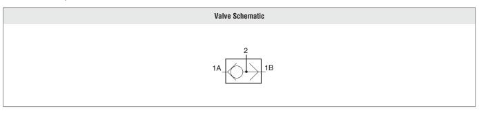
ROSS shuttle valves or double check valves have two inlets and one outlet. The first inlet to be pressurized is connected to the outlet, and the second inlet is then closed. Thus, a pneumatic device connected to the shuttle outlet can be operated by either of two control valves connected to the shuttle inlets. Automatically blocks one inlet passage when pressure is applied to the second inlet. Pressure to either inlet is channeled to one outlet port.
