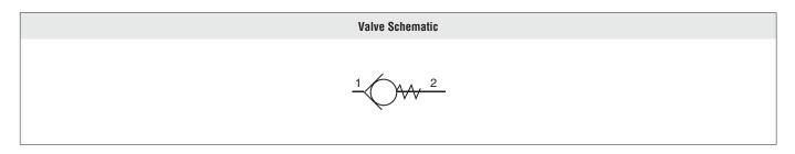
ROSS check valves are self-actuating and designed to provide free air flow in one direction, and to be closed to flow in the opposite direction.
