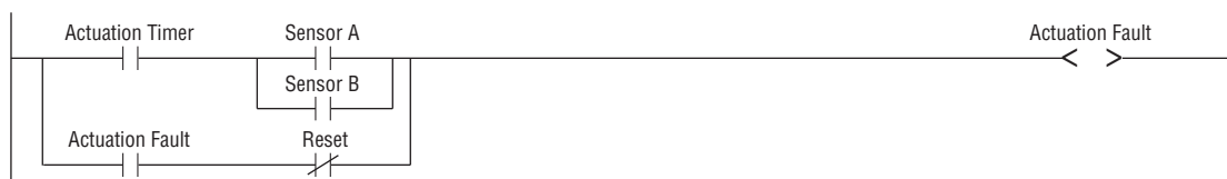
Actuation Fault Monitoring Ladder Logic Example
