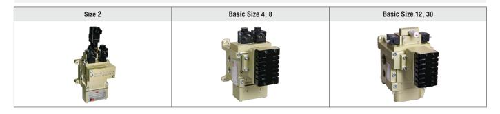
The DM<sup>2®</sup> Series D double valve is a patented 3/2 normally closed valve (with an intermediate, lockout position) distinguished by SERPAR<sup>®</sup> Crossflow passages with poppet and spool valving on the main valve stems. This arrangement provides the valve's outstanding flow characteristics and an integrated monitoring capability with total memory. The valve provides dynamic monitoring and dynamic memory.
