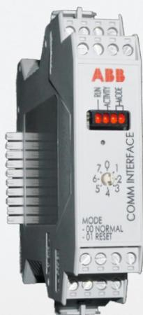
The 2100421 TFIO module is a software configurable serial interface capable of communicating with RS-232, RS-422 or two-wire RS-485 devices at baud rates from 300-38,400 bps.
