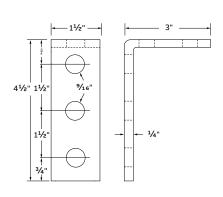
Can also be used as side-beam connector to suspend ½" hanger rod. ¼" steel. 39 lbs/C.
