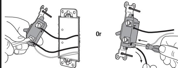
**Screw Terminals:** Turn screws counterclockwise to loosen.
