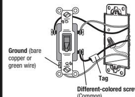
**3-Way Circuit:** Insulated wires connected to three screws: One of these wires is connected to a screw of a different-color. **TAG** this wire to identify it when wiring. Follow: **3-Way Wiring** when completing step 6.
