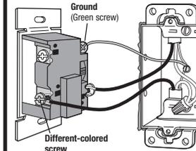
**Helpful Hint:** If you are replacing a single-pole switch with a 3-way or single-pole/3-way dimmer, the screw on the same side as the different-colored screw is not used. Tighten the screw securely.
