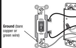
**Single-Pole Circuit:** Insulated wires connected to two screws of the same color: Replace with a single-pole or 3-way dimmer. Follow: **Single-Pole Wiring** when completing step 6.
