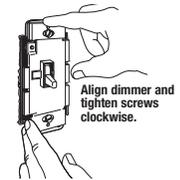
Align dimmer and tighten screws clockwise.
