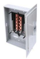
SIEMENS LOW VOLTAGE PL SERIES LOAD CENTER. MAIN LUG WITH 20 1-Inch Spaces ALLOWING MAX 20 CIRCUITS. 1-PHASE 3-WIRE SYSTEM RATED 120/240V(125A) 100KA INTERRUPT. SPECIAL FEATURES: COPPER BUS, INTERCHANGEABLE MAIN, GRAY TRIM, NEMA TYPE1 ENCLOSURE FOR INDOOR USE. REPLACED BY PN2020L1125C. AVAILABLE 4/1/2020
