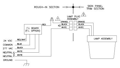
Figure B 277V WIRING F.I. OPTION
