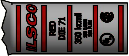
DETAIL B TOP AND BOTTOM INK MARKINGS ARE IDENTICAL INK COLOR: RED PER SPEC #: F921
