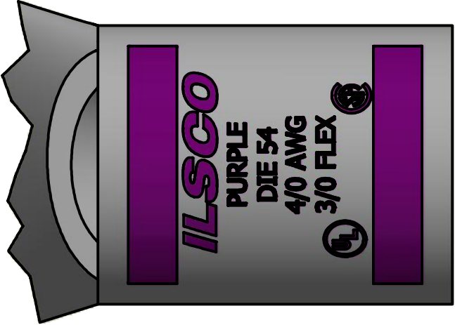
DETAIL B, SCALE 3 : 1 TOP AND BOTTOM INK MARKINGS ARE IDENTICAL INK COLOR: PURPLE PER SPEC #: F921
