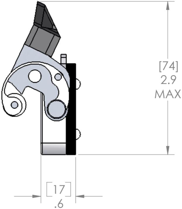
SEAL RATING OF IP 65 ONLY ACHIEVED WHEN FULLY LATCHED TO MATING BASE AND WITH AN APPROPRIATE SEALING GLAND INSTALLED
