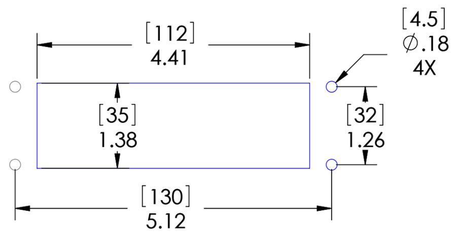
These devices shall be mounted on enclosures having adequate strength and thickness and with adequate spacing provided. Seal rating is based on mounting to a surface that is clean, flat and smooth.
