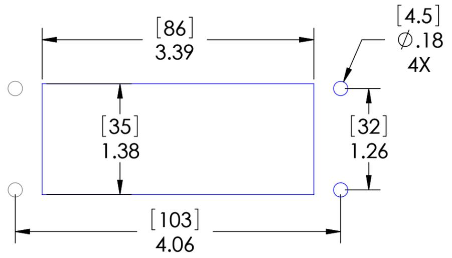
These devices shall be mounted on enclosures having adequate strength and thickness and with adequate spacing provided. Seal rating is based on mounting to a surface that is clean, flat and smooth.
